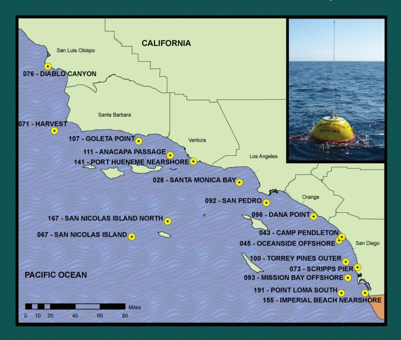
Buoy measures wave height, wave direction, wave period and sea surface temperature. The data are broadcast on the NWS Marine Weather Channel. Data are also **updated every 30 minutes** on the web at **http://cdip.ucsd.edu** (click on RECENT).
