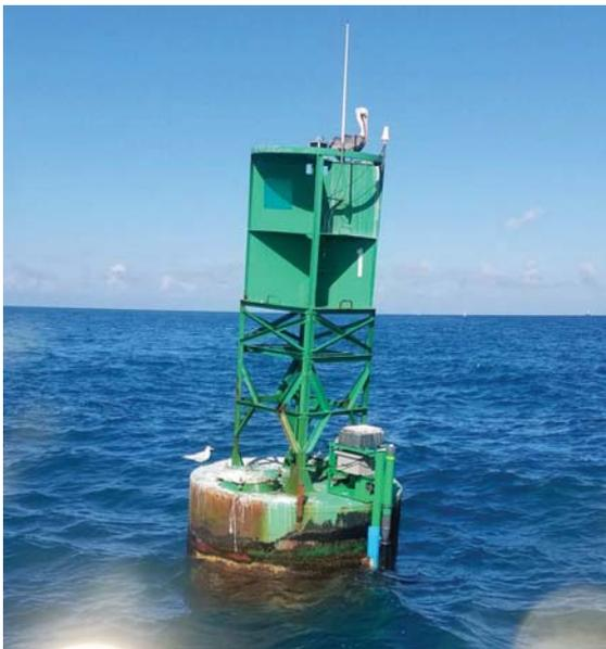
Fig. 3. iATON ADCP and Iridium satellite data telemetry system attached to a standard USCG Aid to Navigation (ATON) buoy in the Miami ship channel as a component of Miami PORTS®. (Photo credit M. Luther)
