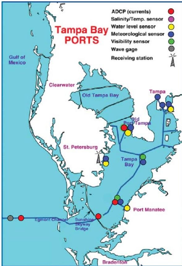
Fig. 2. Map showing TB-PORTS observing sites. Thin blue line shows main ship channel.
