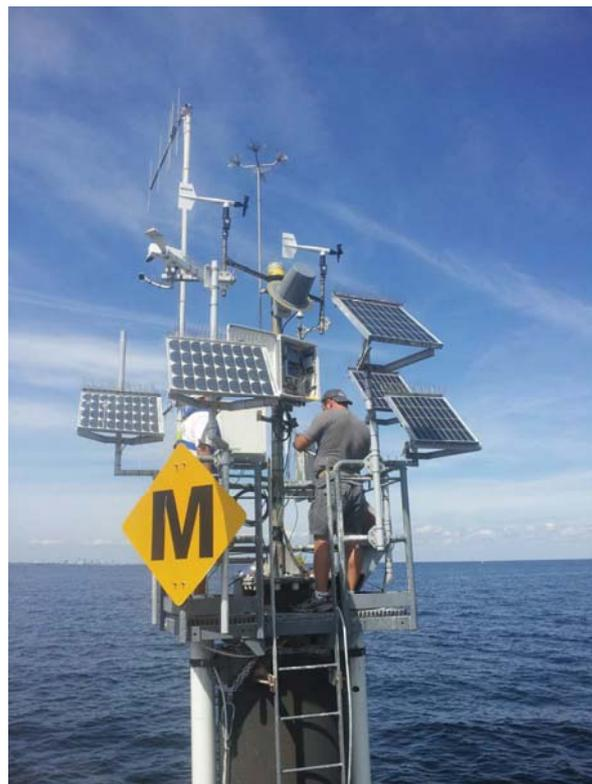
Fig. 4. TB-PORTS instrumented tower at Middle Tampa Bay. This site houses dual RM Young wind monitors, air temperature/relative humidity, barometric pressure, visibility (fog), and ADCP currents as components of TB-PORTS. Additional sensors for other programs are mounted on the tower as well. Visibility sensor is to the upper-left of the photo. (Photo credit M. Luther)
