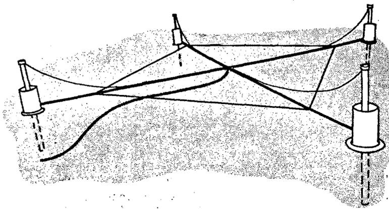
SLOPE ARRAY FOR MEASURING WAVE DIRECTION
