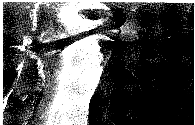
Figure 1. Oblique aerial photograph of the Tijuana River inlet at low tide on December 21, 1987. The inlet has a wide, deep channel following high storm runoff and spring tidal conditions. Note the unrestricted slough channels and deltaic deposits on either side of the mouth.
