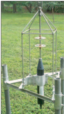
MAVS-3WTG Directional Wave and Tide Gauge
