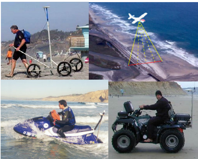
CDIP Survey Methods. Clockwise from upper left: Dolly; Airborne LIDAR; JetSki; ATV
